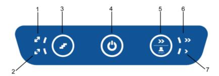
1: Multi-step mode - 2: Single-step mode - 3: Single/Multi-step button - 4: ON/OFF button / status display - 5: Speed button / Stair light - 6: Speed fast display - 7: Speed slow display
