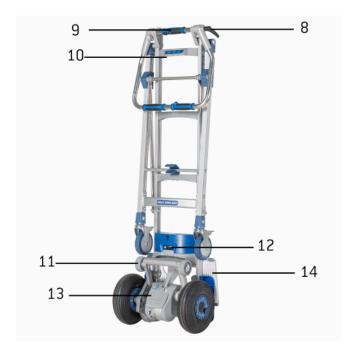
1: Up button - 2: Upper handle - 3: Frame - 4: Dolly kick - out fixation - 5: Dolly kick - out - 6: Quick-change battery - 7: Main wheels - 8: Locking lever - 9: Cross tube handle - 10: Control unit - 11: Swing arm - 12: Charge level indicator - 13: Safety flap - 14: Lifting unit
