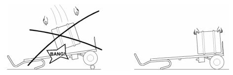
In the beverage industry drums are sometimes directly thrown from the truck onto the hand truck instead of a rubber pad or old tyre.
