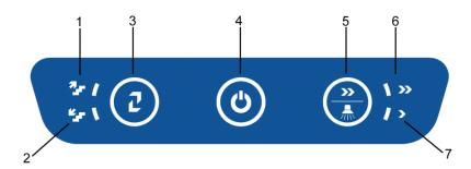
1: Up indicator - 2: Down indicator - 3 Up/Down button - 4: ON/OFF button / Status indicator - 5: Speed button / Stair light - 6: Speed indicator fast - 7: Speed indicator slow
