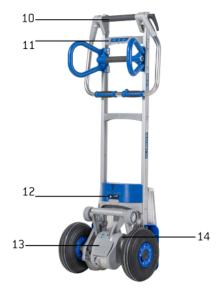
1: Up button - 2: Upper handle - 3: Frame - 4: Locking lever - 5: Lower handle - 6: Quick-change battery - 7: Swing arm - 8: Main wheels - 9: Bucket - 10: Cross tube handle - 11: Control unit - 12: Charge level indicator - 13: Safety flap - 14: Lifting unit
