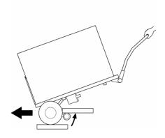
Under normal operating conditions, with the load in a well-balanced position, the moving support arm is always clear of the underside of the upper step (see chapter 4.2). If the LIFTKAR is laid back too far, the support arm will be tripped by touching the tread it is on, causing it to rotate under the upper tread. The electronics will go into overload mode and will need to be reset.
