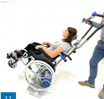
11 Tilt the PT back (into the balanced position), and then off you go.
