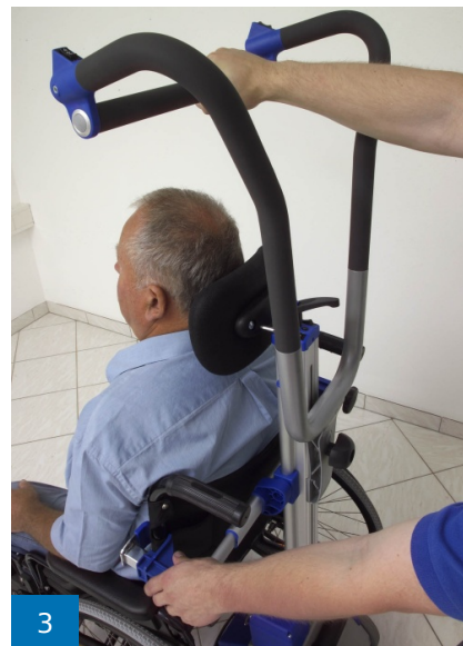
3 Now release backrest clamp on the other side
