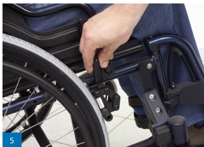
5 Release wheelchair brakes and move clear of PT
