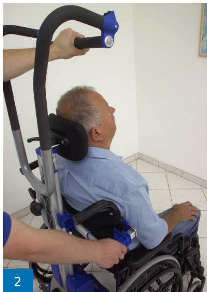
2 Tilt PT forwards with one hand and release backrest clamp on one side with the other hand
