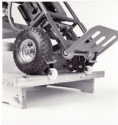
LIFTKAR braked at the step margin
