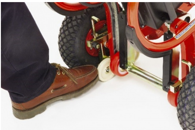
Push the back wheel of the brake forward
