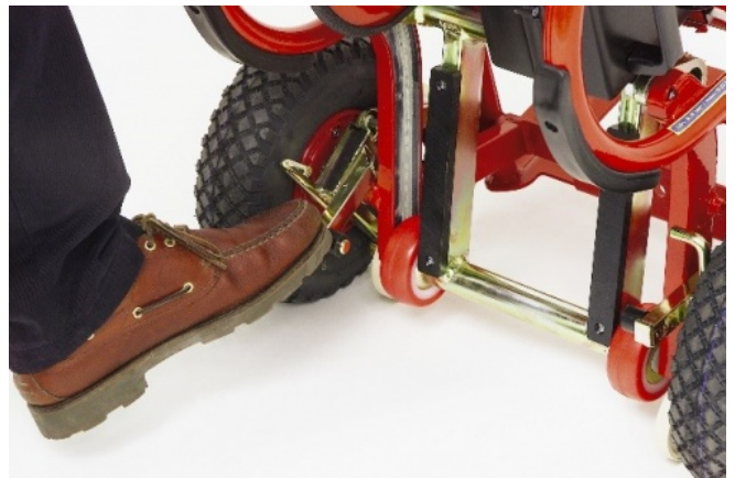
Turning further by foot or hand to neutral position.
